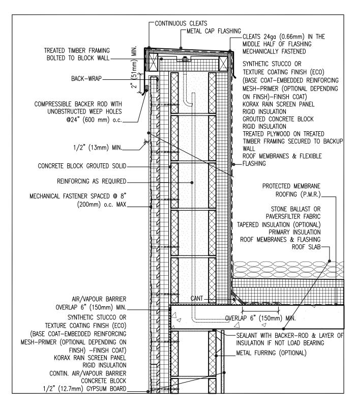
Synthetic Stucco or Texture Coating \ Concrete Block Wall Detail @ Parapet
